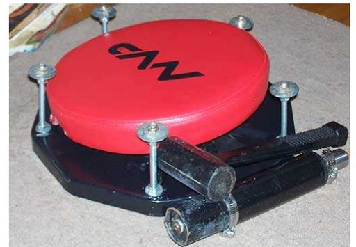
Assembled, the stool can adjust from about 15" to 20". That's only a few inches, but its just enough to account for the movement of the telescope. Including the mallet, it disassembles into four pieces and can be stored in my tote with my eyepiece case, books and so-on.
