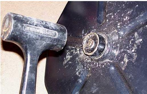
I placed the bottom clamp so that the stool sticks together, and it comes off with a gentle "tap" from a 2lb mallet. (Mine looks a little beat up because I've had mine out and "disassembled" without the handiness of a mallet, so a rock had to suffice)
