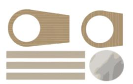
Cut the corrugated cardboard into faceplates, (right) allowing one side to be extended past where the eyepiece would sit in the telescope. This will act as a shade to the viewer's eyes while looking through the eyepiece. Note that only one of the two faceplates need be lengthened.
