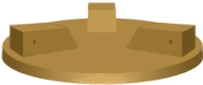
Looking at the tabletop upside-down, we see the leg brackets attached. Attach each block with 2 screws through the tabletop, and be sure to glue the blocks to the tabletop. This connection must be absolutely rock-solid.
